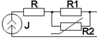
9. Find the power of the feed source, if resistor VAC  $R_2 U_2=5 \cdot (I_2)^2$ ,  $R=R_1=10$  Ohm, resistor current  $R_1 I_1=2$  A.
