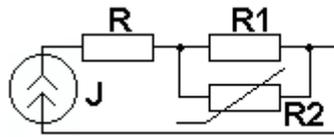
15. Find the applied voltage  $U$ , if resistor  $R$   $U_2 = 5 \cdot (I_2)^2$ ,  $R = R_1 = 10 \text{ Ohm}$ , drop voltage on resistor  $R_1$   $U_1 = 40 \text{ V}$ .
