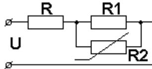
2. Find the value of static resistance  $R_2$  in working point, if resistor VAC  $R_2$   $U_2=5 \cdot (I_2)^2$ ,  $R=R_1=10$ , Ohm, resistor current  $R_1$   $I_1=4$ , A.
