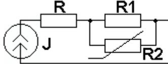
11. Find the value of nonlinear element dynamic resistance in working point, if resistor VAC  $R_2 U_2=5 \cdot (I_2)^2$   $R=R_1=10$  Ohm, resistor current  $R_1 I_1=2$ , A
