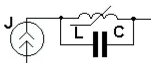
10. Find the capacity value C, at which in point  $U=10 \text{ B}$ , appears phenomenon current ferroresonance, if  $I_L=0.02 \cdot (U)^2$ ;  $f=50 \text{ Hz}$ .
