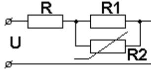
3. Find the value of dynamic resistance  $R_2$  in working point, if resistor VAC  $R_2$   $U_2=5 \cdot (I_2)^2$   $R=R_1=10$  Ohm, resistor current  $R_1$   $I_1=4$ , A.
