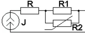
10. Find the value of nonlinear element static resistance in working point, if resistor VAC  $R_2 U_2=5 \cdot (I_2)^2$   $R=R_1=10$  Ohm; resistor current  $R_1 I_1=2$  A.
