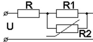
4. Find the value of nonlinear element current, if resistor VAC  $R_2$   $U_2=5 \cdot (I_2)^2$   $R=R_1=10$  Ohm,  $U=70$  V.
