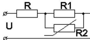
5. Find the value of nonlinear element dynamic resistance in working point, if resistor VAC  $R_2$   $U_2=5 \cdot (I_2)^2$   $R=R_1=10$ , Ohm;  $U=70$  V.
