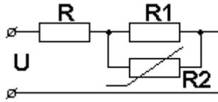
8. Find the drop voltage on resistor R, if VAC  $R_2 U_2=5 \cdot (I_2)^2$ ,  $R=R_1=10$  Ohm, resistor current  $R_1 I_1=2$  A.
