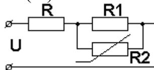
7. Find the power of the feed source, if resistor VAC  $R_2$   $U_2=5 \cdot (I_2)^2$ ,  $R=R_1=10$  Ohm, resistor current  $R_1$   $I_1=4$  A.
