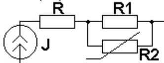
14. Find the value of nonlinear element dynamic resistance in working point, if resistor VAC  $R_2 U_2=5 \cdot (I_2)^2$   $R=R_1=10$  Ohm;  $J=4$  A.
