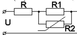
6. Find the value of nonlinear element static resistance in working point, if resistor VAC  $R_2$   $U_2=5 \cdot (I_2)^2$   $R=R_1=10$  Ohm;  $U=70$  V.
